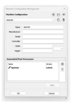
4) Make sure all instances of VCarve are closed before opening up a new window. Go to the top menu bar and open Machine > Machine Configuration...
